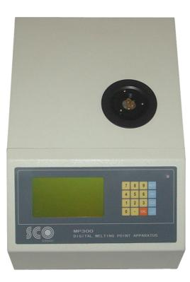
High quality microprocessor instrument for precise measurement of melting points of solid Materials for max. melting point of 300°C.
