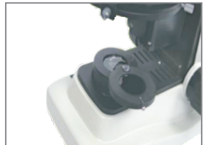
Polarizer can be swung out of optical path. 6v20 W halogen lamp illumination brightness adjustable
