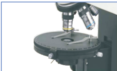
Revolving round stage \varnothing 145mm, 360^\circ rotatable and graduated in 1^\circ increments, minimum resolution 6^\circ , when using vernier scale
